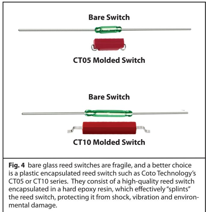
**Fig. 4** bare glass reed switches are fragile, and a better choice is a plastic encapsulated reed switch such as Coto Technology's CT05 or CT10 series. They consist of a high-quality reed switch encapsulated in a hard epoxy resin, which effectively "splints" the reed switch, protecting it from shock, vibration and environmental damage.
