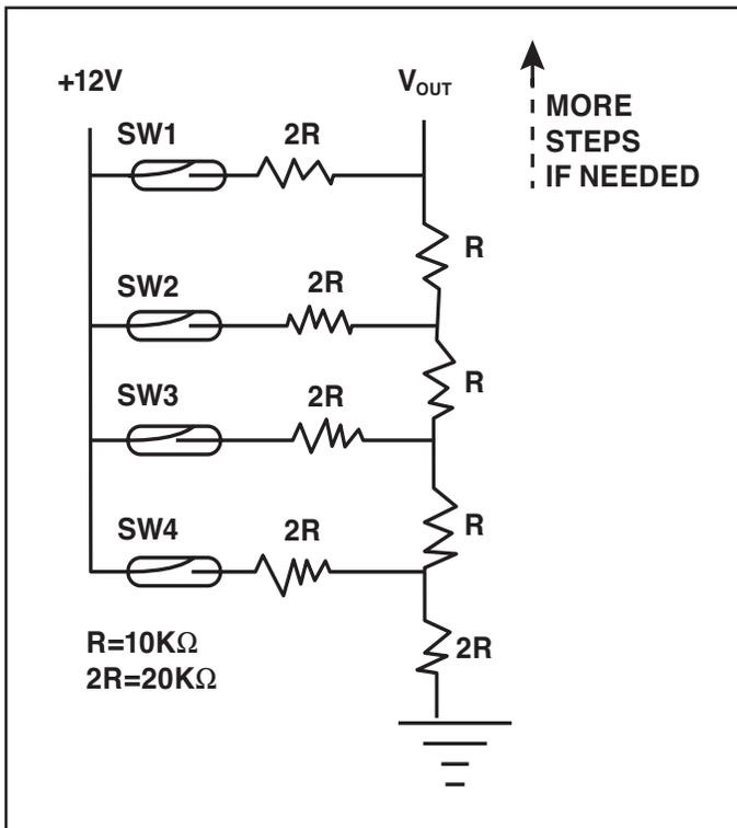
Fig. 2 Reed switch - R 2R resistor ladder diagram.
