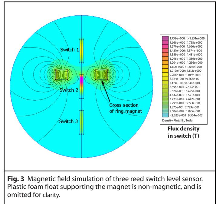
Fig. 3 Magnetic field simulation of three reed switch level sensor. Plastic foam float supporting the magnet is non-magnetic, and is omitted for clarity.
